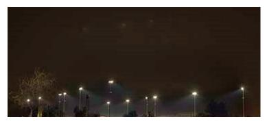
Downward-directed, shielded site lighting no higher than noise wall
