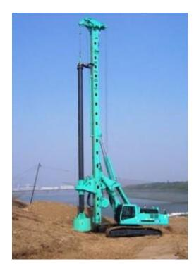
Noise reduction measures including use of pile drilling instead of pile driving where possible
